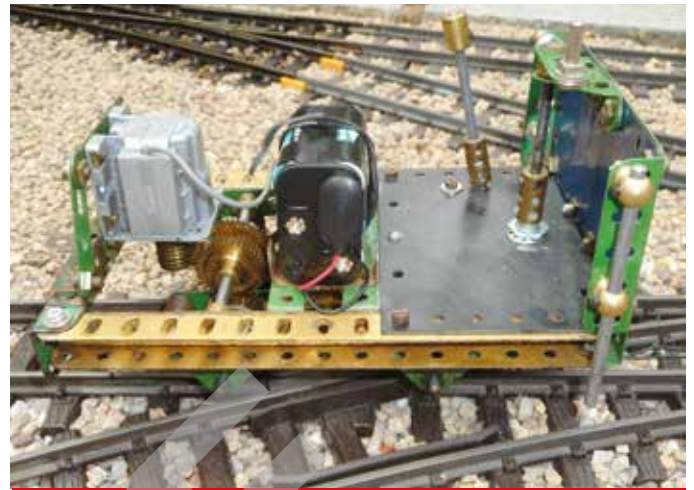
■ The loco's insides. The body simply lifts off for access to the batteries. I made a replacement cab floor from 2mm styrene sheet to avoid short circuits - delicate electronics and metal Meccano do not mix.
