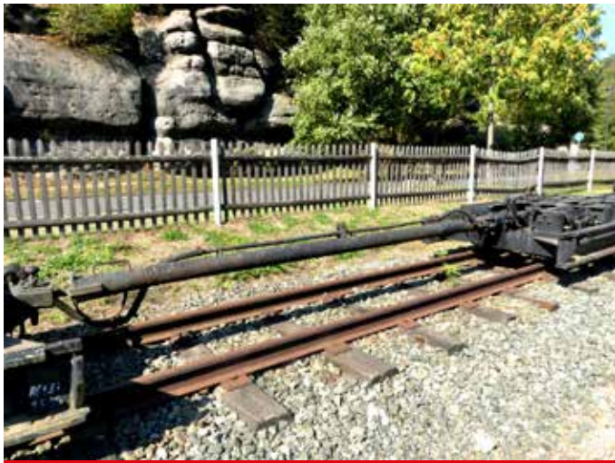
■ Coupling bar between two RWs. Note the air pipe - a detail not included in the LGB model but is included in the Magnus one. The Magnus model is hand made, superbly detailed, and expensive and no longer available new. These RWs at Obyin were on display but looked like they hadn't been used in quite a while, poss not serviceable.
